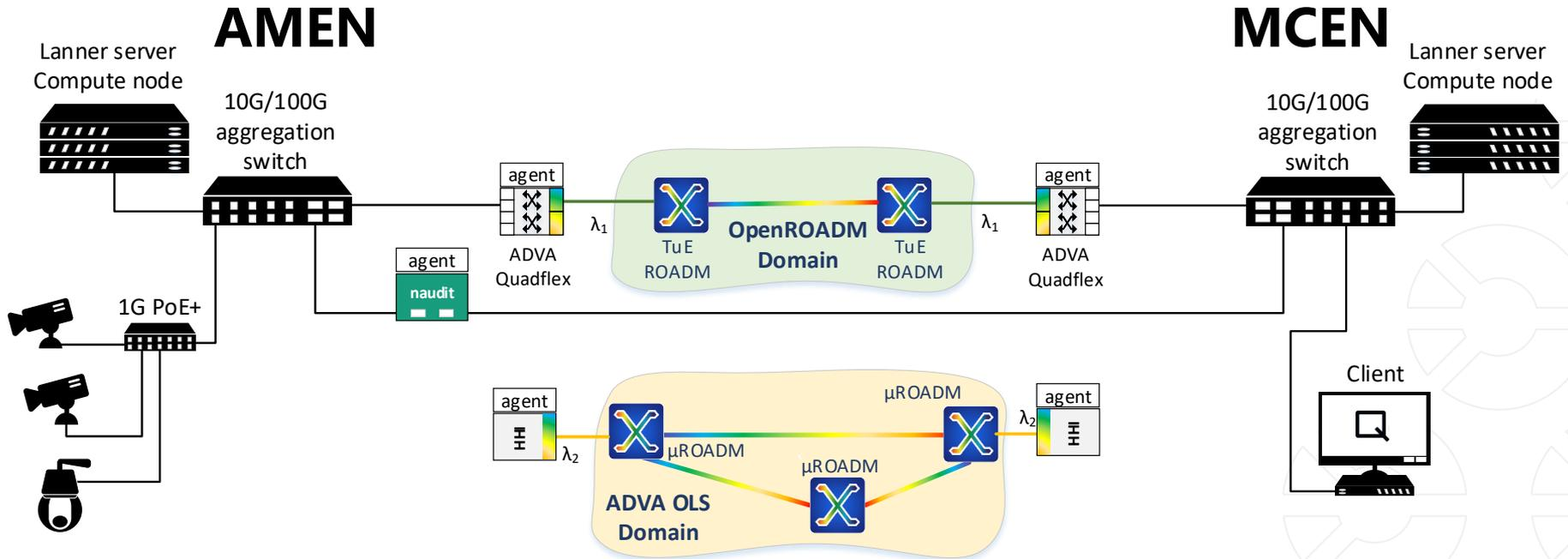
Compute nodes and cameras are connected via switches
