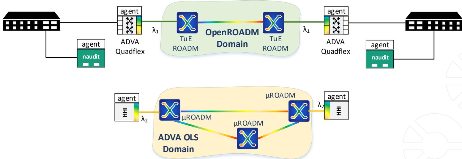
Active and passive probes for latency measurements and channel monitoring
