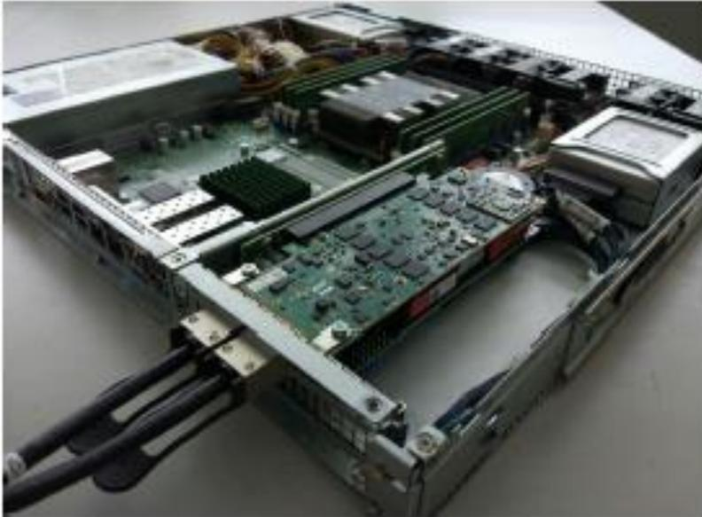
Fig. 2 Active network probe implemented in a small factor server. FPGA is placed in the bottom corner, with both QSFP28 interfaces connected. Management interfaces are on the left.
